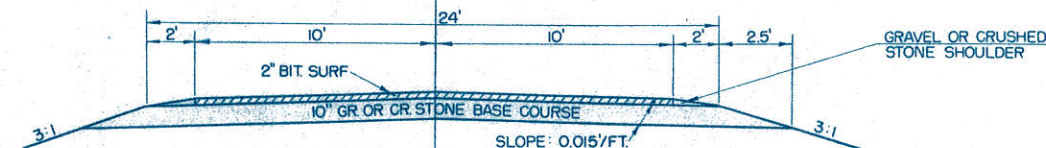
TYPICAL SIDE ROAD SECTION
