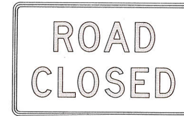
R11-2 48"(121.9 cm) x 30"(76.2 cm) Black Lettering on Reflective White Background Letter Series "D" Letter height 8" (20.3 cm)
