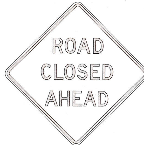
W20-3 48"(121.9 cm) x 48"(121.9 cm) Black Lettering on Reflective Orange Background Letter Series "D" Letter height 7" (17.8 cm)
