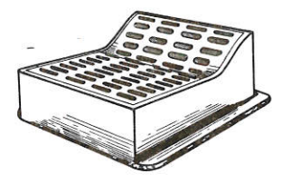
TYPE "F" (Approximate Weight 850 lbs.) Frame 515 lbs. Back grate 160 lbs. Front grate 175 lbs.
