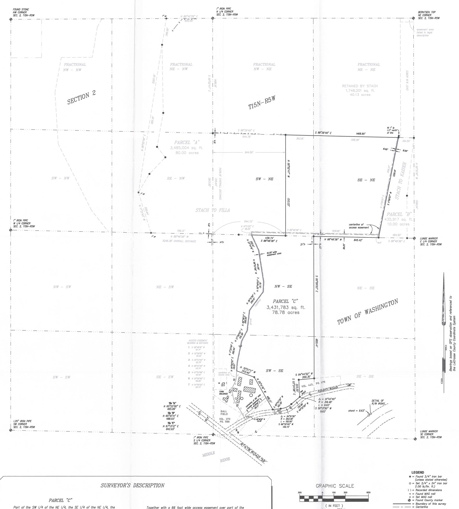
Part of the SW I/4 of the NE I/4, the SE I/4 of the NE I/4, the NW 1/4 of the SE 1/4 and the SW 1/4 of the SE 1/4, Section 2, TI5N-R5W, Town of Washington, LaCrosse County, Wisconsin described as follows: Commencing at the South 1/4 corner of Section 2, thence N 67°13'12" E 842.93 feet to the northerly right-of-way line of County Road "JB" and the point of beginning: thence N 29°41'16" W 486.21 feet;
